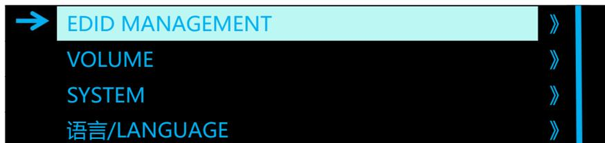
2. Press the knob and enter to input source need to be changed in sub-menu of EDID, the input listed can be changed, we will use HDMI2.0 as a example.
