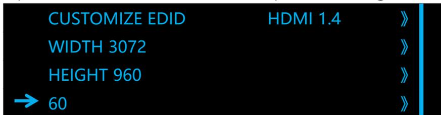
5. After step 4, return to the menu and overview the status. (pls note that some PC will work successfully after remove and re-connect the input )
