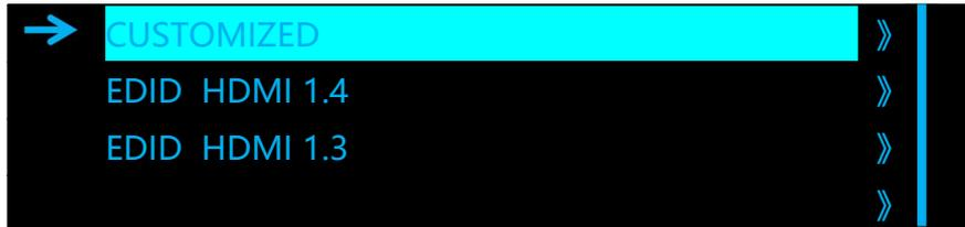
4. After step 3 is done, rotate the knob to input and change the EDID
