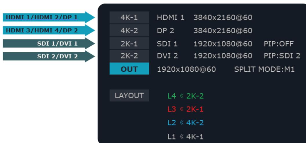
Note: Switching Input channel within input module will take 1-2s to proceed.
