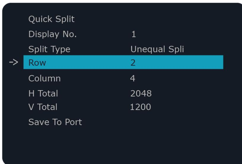
2) The required parameters will show automatically. Fill in the related parameters and click Save To Port to apply settings.
