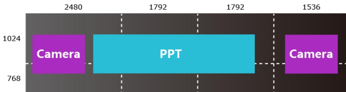
From the configuration, the biggest part for the screen is 2048x1024. Then output resolution need no less than 2048x1024.
