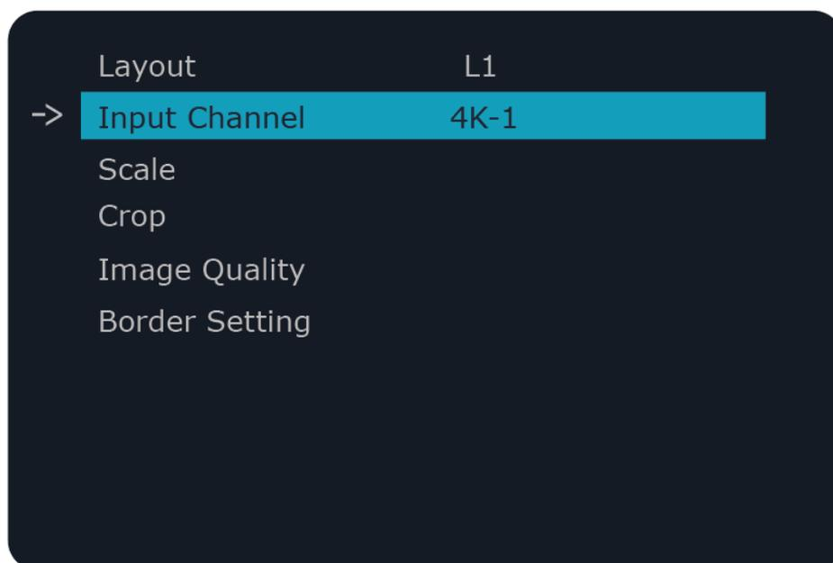
2) For L1 & L2 the input channel can be 4K-1/4K-2. Push knob to arrange proper input channel.
